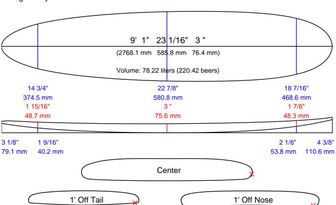
Measurements are center, one foot in and one foot back, over curve.
